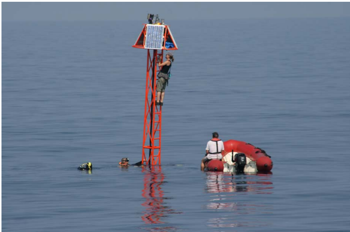
Figure 1. Change of the cable between the Argos beacon on the top of the buoy and the Dacnet.
